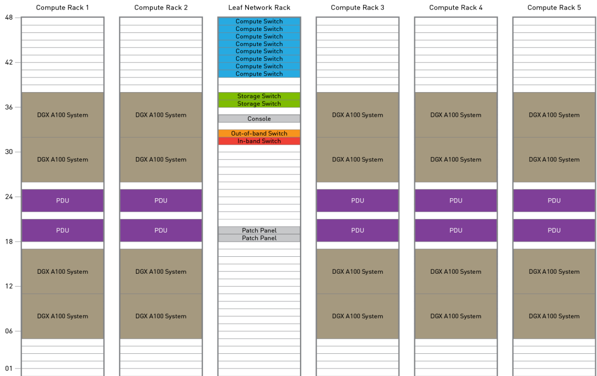
Figure 14. SU rack elevations
